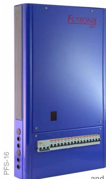
The PFS switching unit is available in 8, 12 or 16 channel formats and is designed for controlling dimmable fluorescent ballasts, curtain/drape/window shade motors and other motorized equipment such as swimming pool covers and sky lights. The unit has motor interlocking, for operating dual-motor curtain and drapes.
